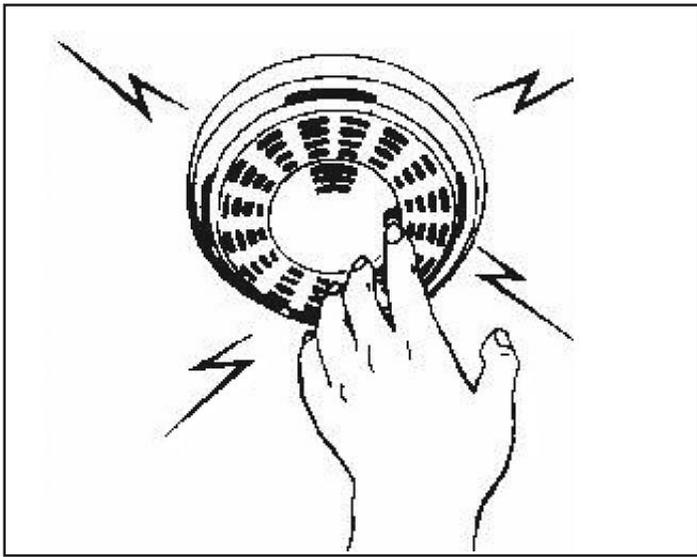
**Figure 2.2.** Smoke Alarm Testing
