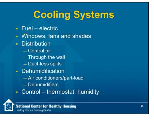
Residential cooling systems are nearly all powered by electricity. There may be one or multiple cooling units. The cool air may be distributed using ductwork or cool air may be blown from the unit directly into the room (window air conditioners and ductless split air conditioners).
