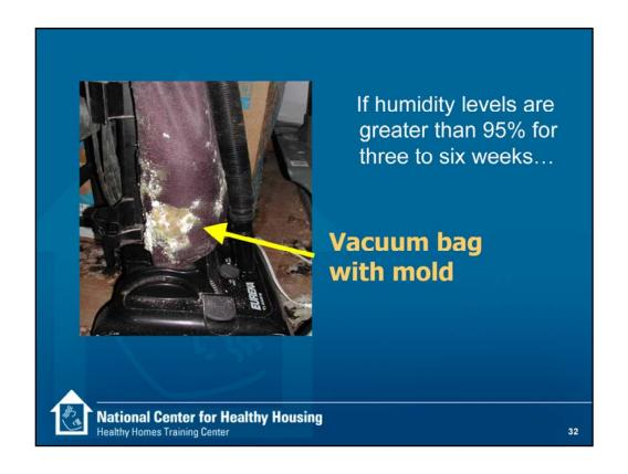
Chronically high humidity can result in mold growth. While it is true that mold spores generally need a small amount of liquid water to germinate and hyphae tips certainly need liquid water to exude enzymes and absorb digested nutrient, it does not take a lot of liquid moisture. At 90% relative humidity an ordinary surface only needs to be 6 degrees F cooler than the air to be at dew point. In a building, it is likely that there are surfaces a few degrees cooler than house air.
