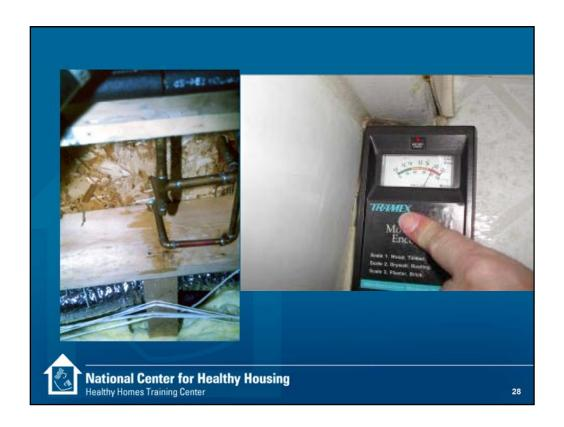
The next category of problem water is plumbing leaks. When plumbing leaks occur, it is best if they are easy to see, easy to repair and do not wet materials that facilitate mold growth or dry slowly. Wet rooms, such as kitchens, baths and laundry rooms, are the places most likely to have plumbing leaks. Always inspect around toilets, tubs, showers, beneath sinks, clothes washers and dishwashers.
