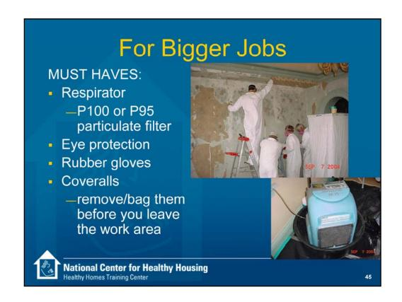
As the size of the area needing remediation increases or if demolition is involved, the chance of larger exposures increases and more worker protection and containment are advised.<sup>[8,9,11]</sup> Quickly drying things out is an important step, because mold will continue to grow as long as there is moisture and nutrient.
