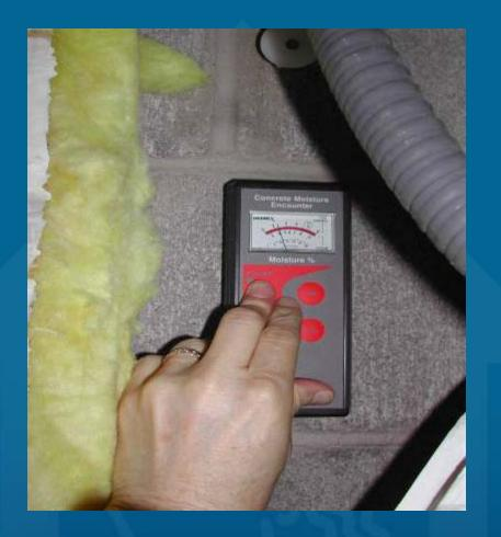
Moisture meters are useful in determining whether a material is wet or not and tracing the source of problem water.
