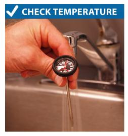
4. If temperature is too low, adjust the thermostat. Repeat until desired temperature is reached.
