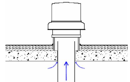
**Figure 7** | Leakage between sheetrock and horizontal take-off duct
