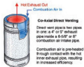
Figure 5.8 Direct Power Vent Increases Energy Efficiency and Helps Avoid Back Drafting Problems
