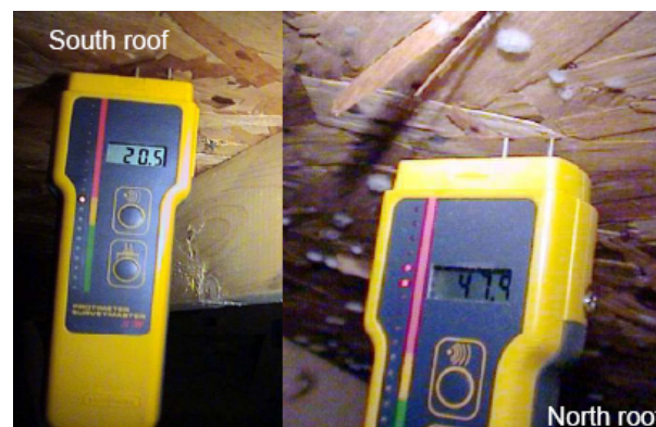
Figure 4.12 Moisture Meters as an Adjunct to Visual Assessment of Moisture Problems
